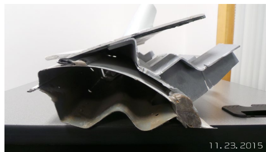
Figure 9. Front cut assembly cross section
