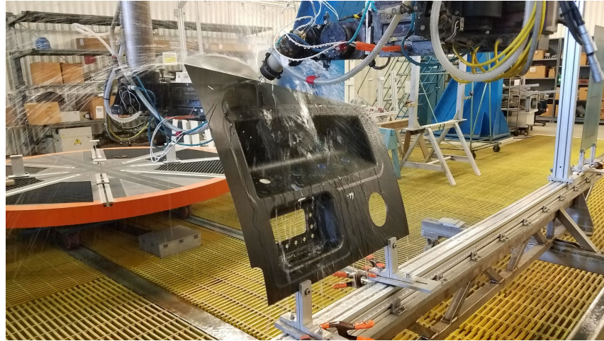
Figure 14. Automated ultrasonic scanning system (AUSS) used for C-scans of challenge parts (RI-RAPM-004).
