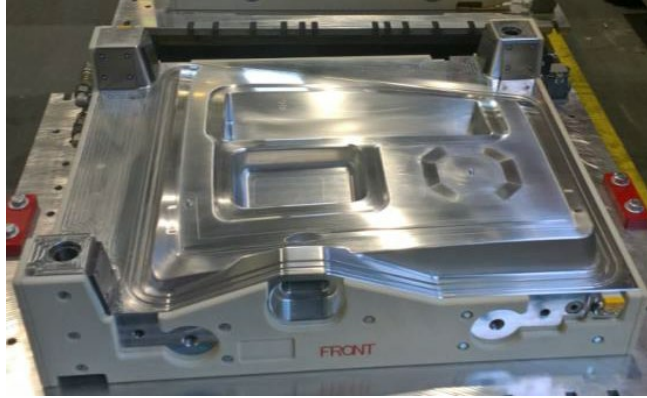
Figure 4. Image of one of the mold faces for the challenge part (RI-RAPM-004), made from A15083.
