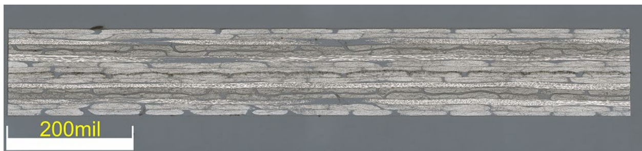
Figure 17. Representative cross section of challenge part taken from pad-up around V-shaped deep-draw section
