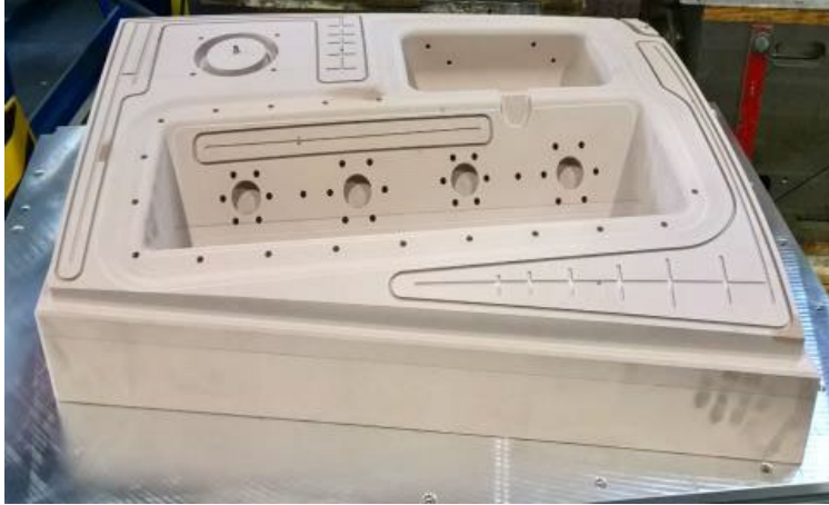
Figure 6. Trim fixture for milling of challenge part (RI-RAPM-004).
