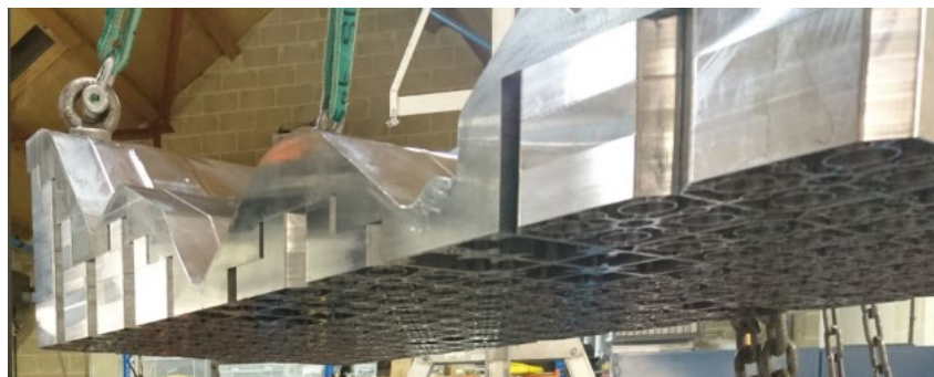
Figure 12. Representation of Building Block and machined mold face. Courtesy of Surface Generation.
