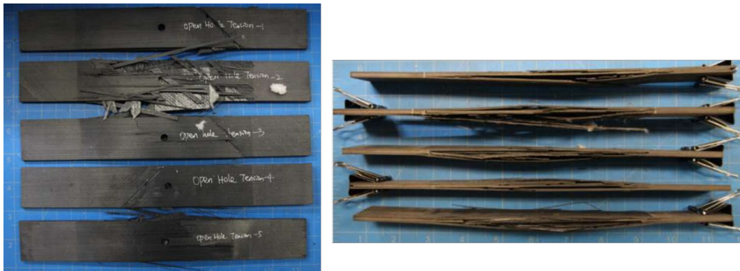
Figure 8. Failure of the Open Hole Tension coupons
