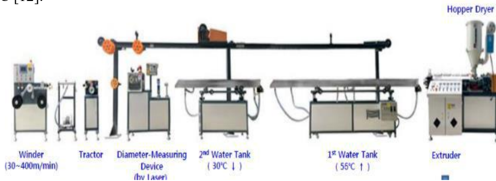
Figure 2. Solid Space extrusion machine setup
