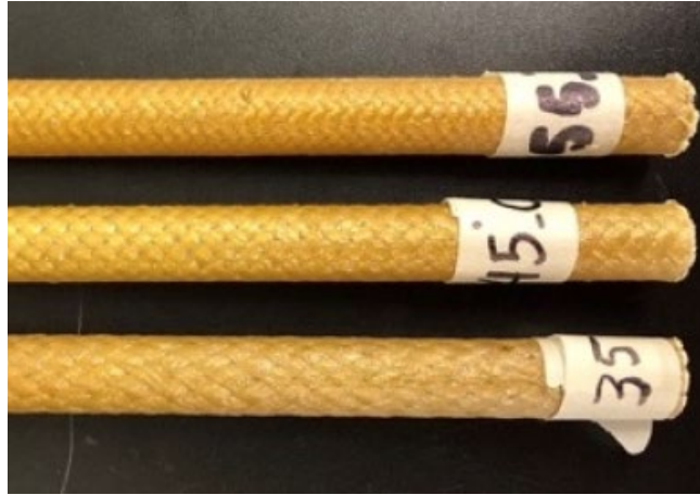
Figure 8: Preform placed on Teflon mandrel before impregnation with resin and hardener.
