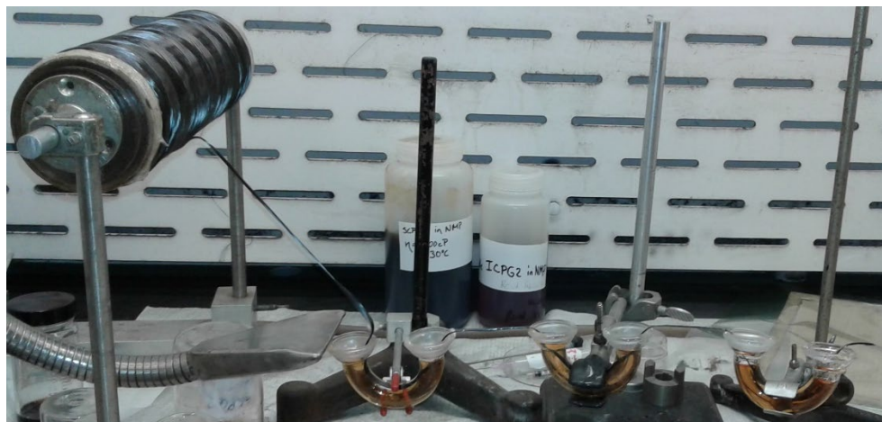
Figure 1 Set up for the wetting and infusion of the fiber tow with polyimide matrix
