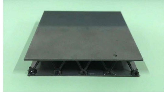
Figure 2. SMA lattice sandwich structure
