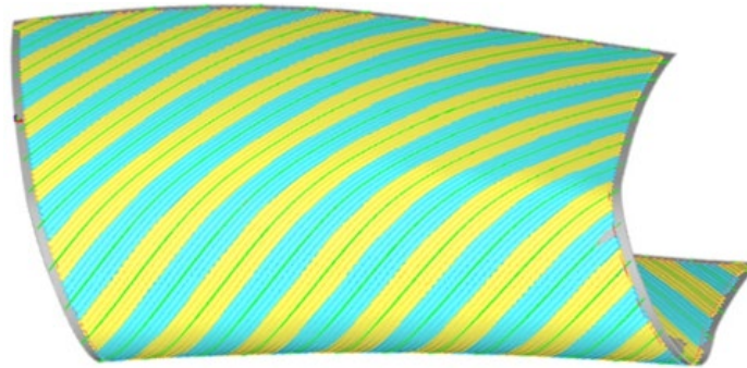
Figure 7. VCP tow paths for a 45° ply.
