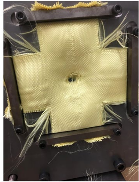
Figure 1. A) Treated aramid fabric sample for tow pullout. B) Tow pullout testing experimental setup. C) Photoresistors recorded signals as projectile exits the barrel. D) Cross-shaped, 4 sided clamped shot aramid fabric.
