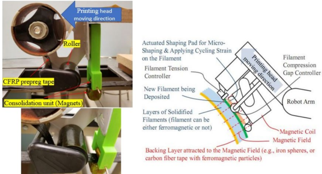
Figure 2. A simplified hand-held printing head designed for this feasibility trial of MCFA-AM (left) and the MCFA-AM printing head schematic described in [31] (right).
