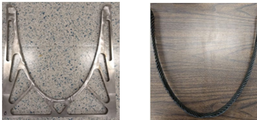
Figure 13. Welded Invar-steel structure (left). CF/Epoxy composite manufactured in the welded invar-steel structure (right).
