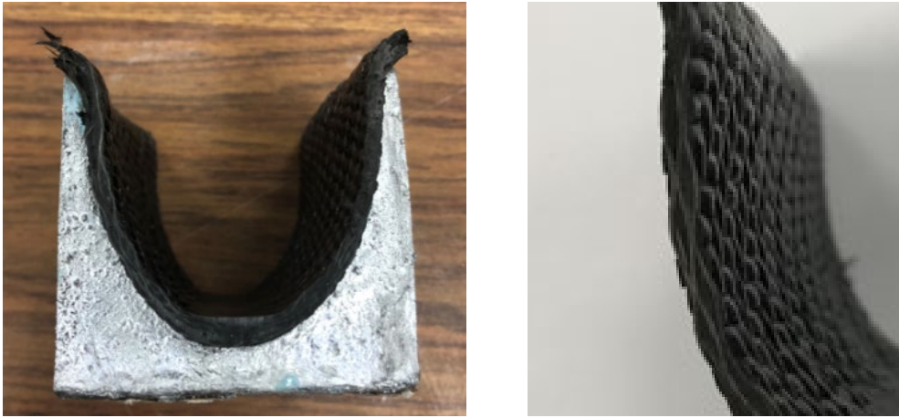
Figure 10. Transformed SLA printed part. Included in the figure, is the manufactured CF/Epoxy composite, as well as a magnification showing the consolidation.
