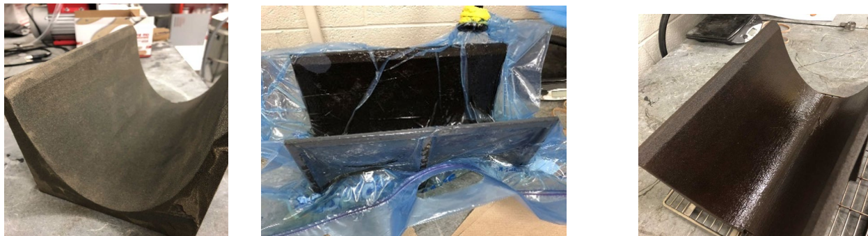
Figure 3. Polymer infiltration process. As-received printed part (left). Resin infiltration under vacuum (center). Final infiltrated part (right).
