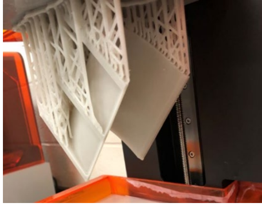
Figure 4. Printed tooling part in a Formlabs 2 unit using a silica ceramic resin.
