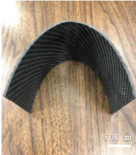
Figure 8. Lead edge composite parts formed on BJB epoxy infiltrated 3D printed ceramic tooling molds. Obtained from the silica sand mold (left). Obtained from the zirconia sand mold (right).
