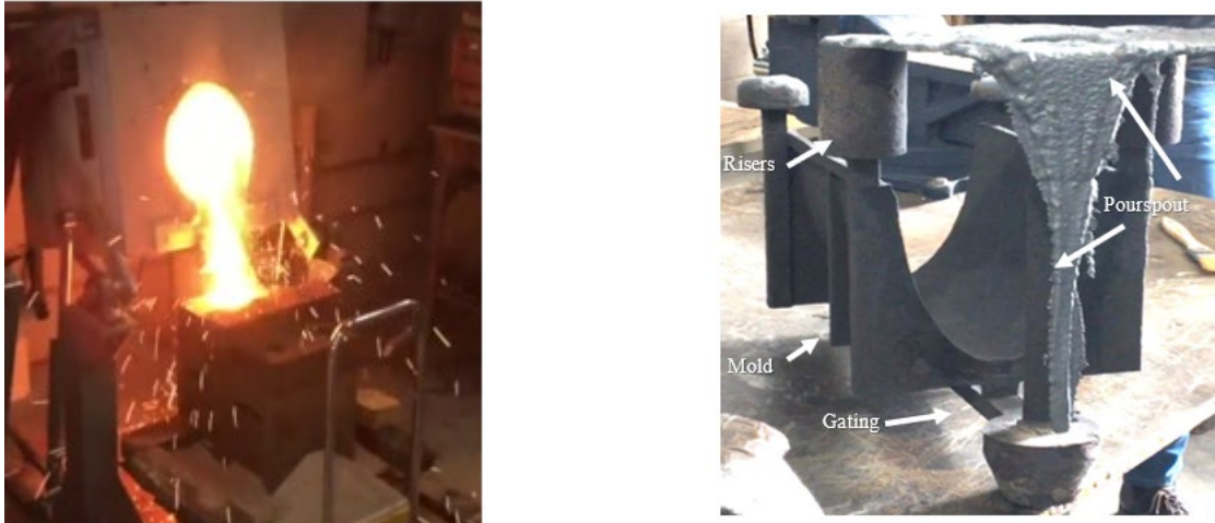
Figure 2. Casting process of Invar-36 (left). Casting part after removing the silica mold.
