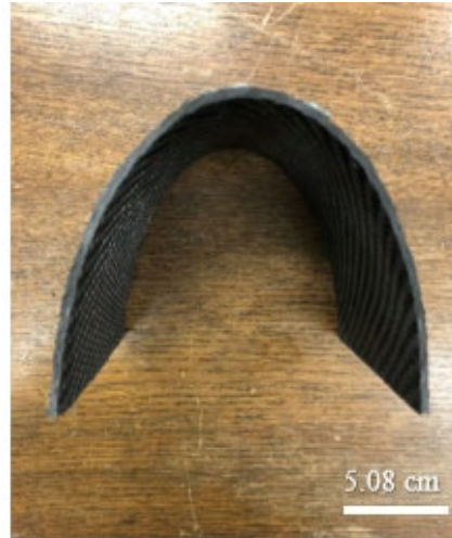
Figure 8. Lead edge composite parts formed on BJB epoxy infiltrated 3D printed ceramic tooling molds. Obtained from the silica sand mold (left). Obtained from the zirconia sand mold (right).
