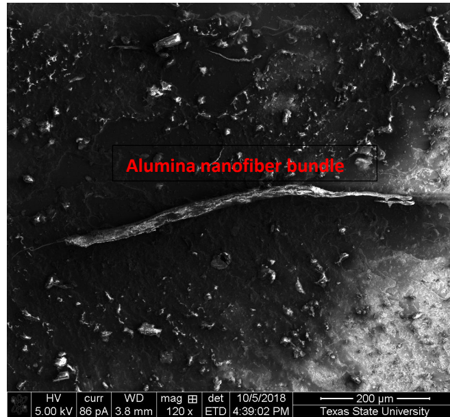
Fig 2: SEM image of alumina nanofiber modified UPE
