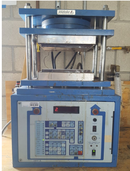
Figure 10 – Composite press The composite materials utilized were cured using the Cal Poly Aerospace Engineering composite press (pictured in Figure 10). The cure cycle for the triaxially woven material can be seen in Figure 11 while the chopped fiber material's is pictured in Figure 12. The shortest cure cycle for the HX42 (Figure 11) was elected to allow for rapid iterating and production.
