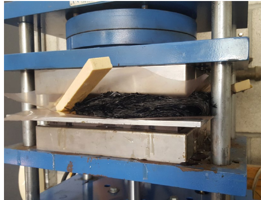
Figure 14 – HDF cure failure
