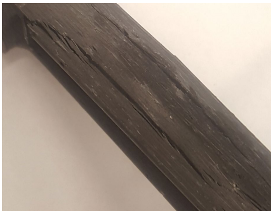
Figure 32 – Chopped rod failure
