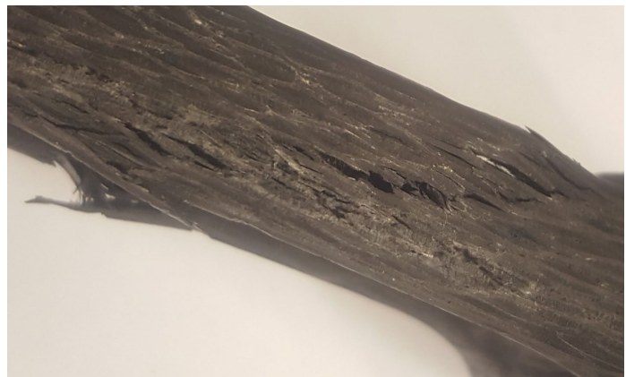
Figure 33 – Woven rod failure
