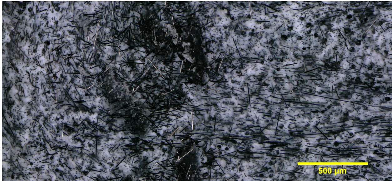
Figure 4. Micrograph of BAAM system bead showing varied fiber orientation
