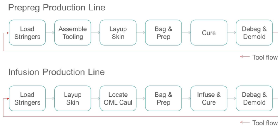
Figure 4. Outline of the prepreg and infusion techniques showing the constituent processes.
