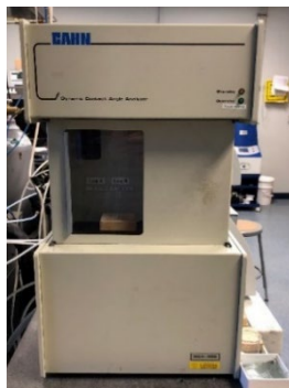
Figure 3: Cahn DCA analyzer used to measure contact angle
