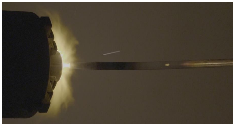
Figure 4. MXB-360 test model undergoing OTB aerothermal testing.
