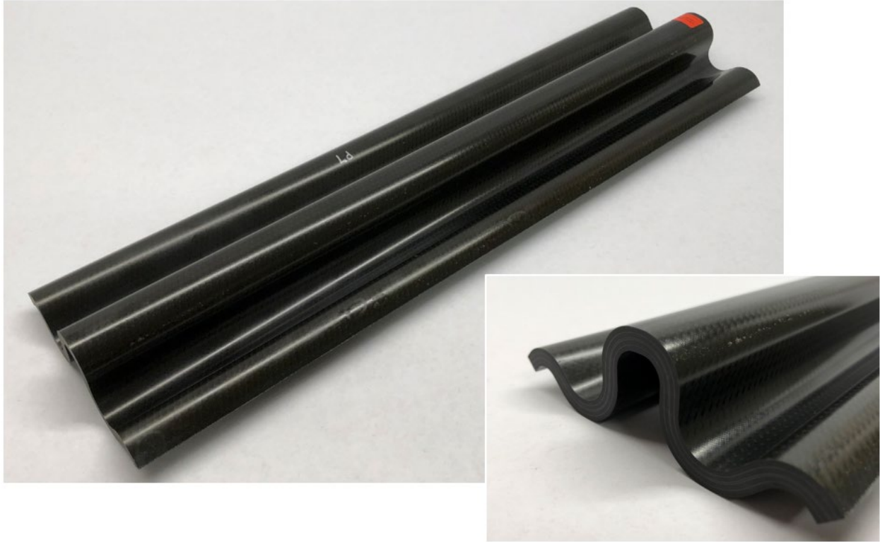
Figure 8 - Completed TS-RAPM-012 Laminate
