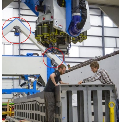
Figure 1. Large-field automatic inspection system mounted to a second gantry over a large AFP cell. Two inspection units are circled in red.
