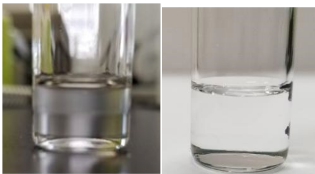
Figure 1. Initial evaluation of silicone solubility in candidate solvent. Left: silicone immiscible in solvent. Right: silicone miscible in solvent.
