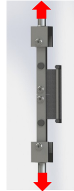
Figure 3. OCT specimen fixture configuration and loading direction; the metal bars clamped to the right side of the specimen limits out of plane bending
