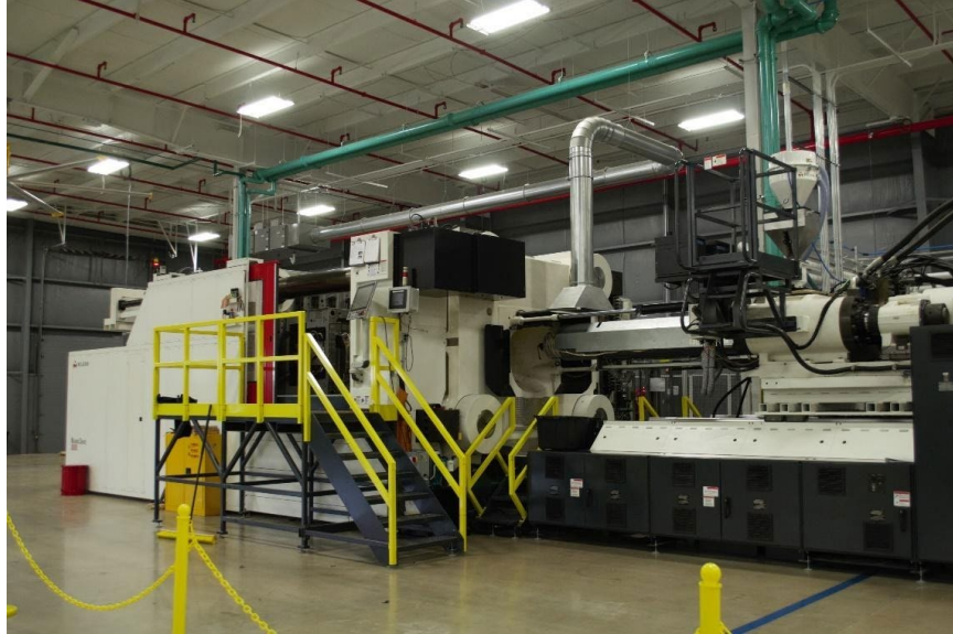
Figure 2: Injection molding machine used to make fenders
