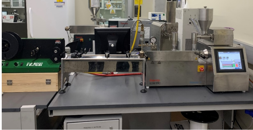
Figure 2. Twin Screw Extruder (11mm diameter)
