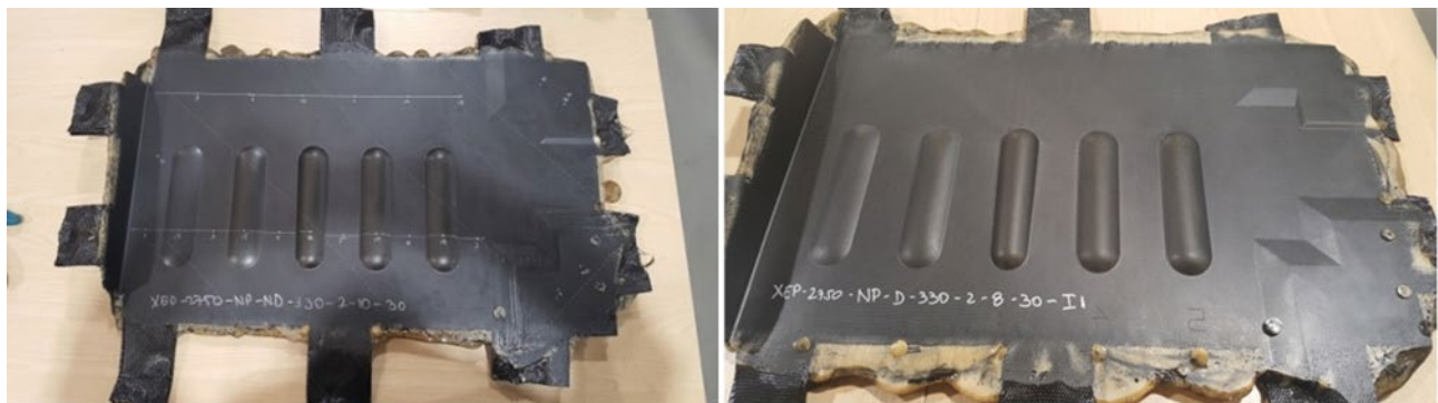
Figure 4. TS-RAPM-009 beaded panel parts after spring-frame molding. Both parts are made using CYCOM® EP2750. On the left, a dwell time of 10 minutes was used. On the right, a dwell time of 8 minutes was used
