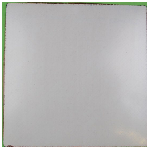
Figure 5. BMI Surfaced CYCOM® 5250-4 Composite Structure (Autoclave Only Cure)
