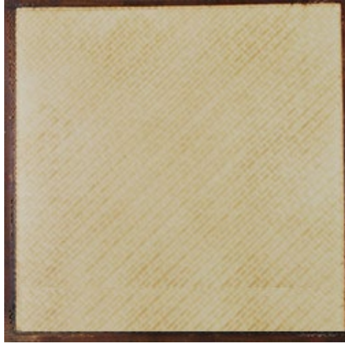
Figure 6. BMI Surfaced CYCOM® 5250-4 Composite Structure (Autoclave + Post Cure)
