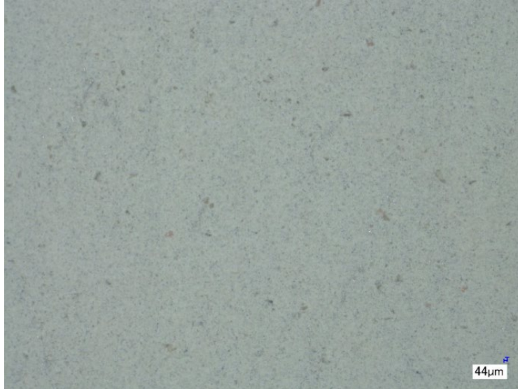
Figure 10. 3D microscope Image of BMI Surfaced CYCOM® 5250-4 Composite Structure (Autoclave Cure)
