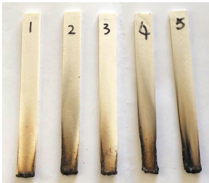
Figure 7. Post-test FFF printed UL94 samples ((material contains 63 wt.% nylon 6/66, 15 wt.% TPE, and 22 wt.% FR).
