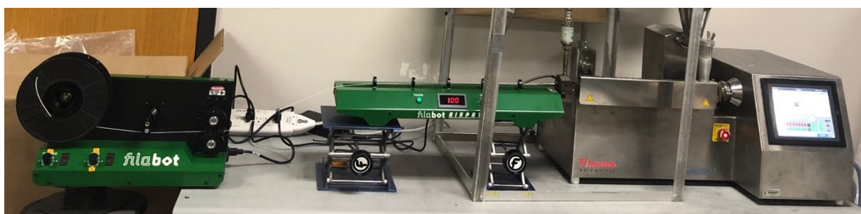
Figure 2. Filament extrusion process equipment (from right to left is Thermo Scientific Parallel Twin Screw Extruder and Filabot Airpath and Filabot Filament Winder).
