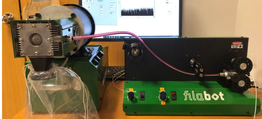
Figure 3. Filament pelletizing process equipment (from right to left is Filabot Filament Winder and Filabot Pelletizer).
