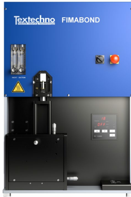
Figure 2. The FIMABOND embedding station of the FIMATEST system. The device is used to prepare the single-fiber composite samples for subsequent pull-out testing.
