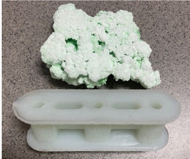
Figure 11: Footstrap Insert from Recovered Thermoplastic Polymer.
